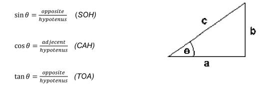
**Example:**  $\theta = 20^{\circ}$  and c = 10 m, solve for **a** and **b**
